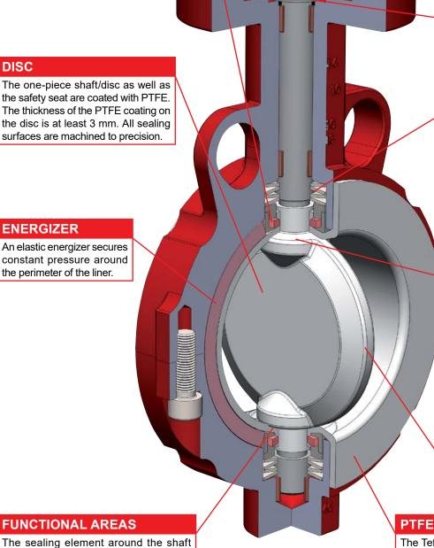
(functional areas) is secured via precise machining and exact alignment of the sealing components.
