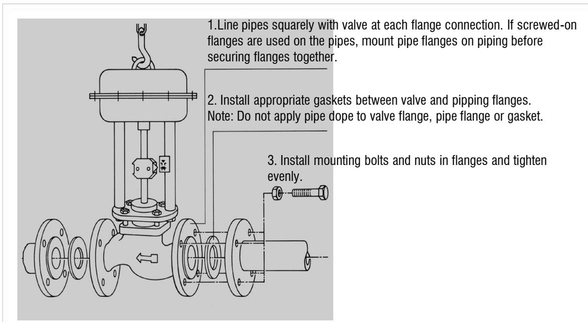
Fig. 1: Installed valve
